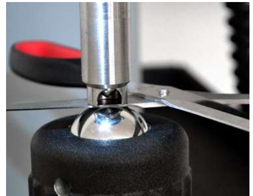
Eyeball anvil. This anvil is used to align slightly tapered samples such as blades. Part No - 900007088
