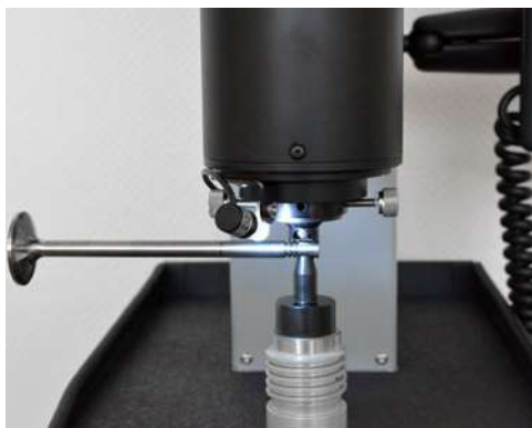
V Anvil shallow 1" [25mm] stem height for small cylindrical parts, such as valves and pins. Part No 900007195
