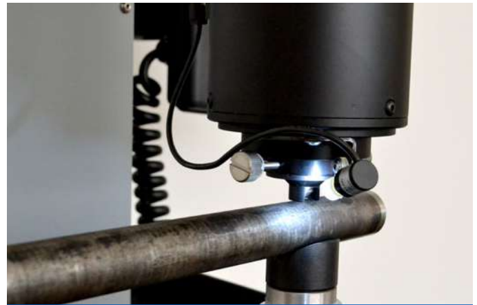
V Anvil standard and clamping device. Part No. 900030797 and W2100CL
