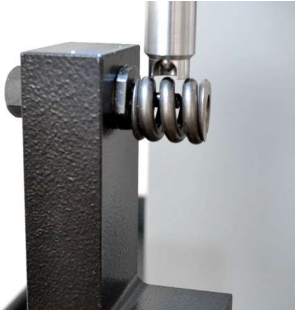
Testing of springs or shells using a gooseneck anvil with mandrels of different diameters. Gooseneck anvil with 0.25" [6,35mm] mandrel. Part No - 900007803
