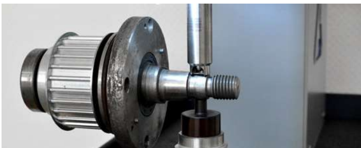
Anvil shallow, clamping device, indenter extension 2". Part No. - 900007388, W2100CL, and W2100E2
